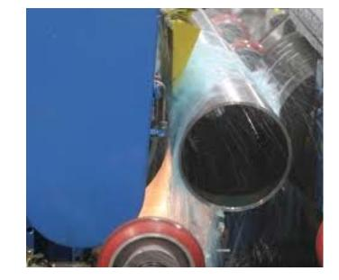
Alliant Metals Inc. is proud to announce the addition of Centerless Grinding to our list of value-added services. Our Cincinnati Twin Grip Centerless Grinder will provide tight tolerance thru-feed grinding for manufacture of parts up to 14 feet long and up to 6 inch in diameter.
